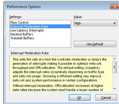
8. Ensure that the **Receive Buffers** setting has the highest possible value.
