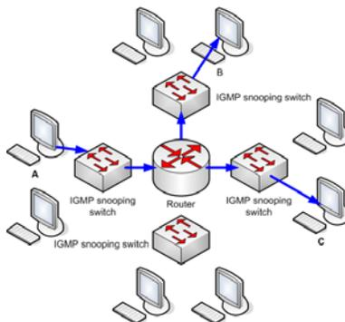
IGMP snooping is disabled by default in LAN switches. To avoid IP multicast flooding problems you must enable IGMP snooping in your Ethernet switch using the managed (or other) interface of your switch.
