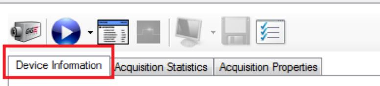
The **Device Information** tab on the right pane displays and allows you to specify basic information about the selected GigE Vision device.
