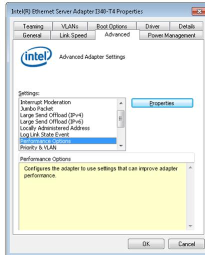
6. In the **Performance Options** window that appears, ensure that **Flow Control** is set to **Enabled**.
