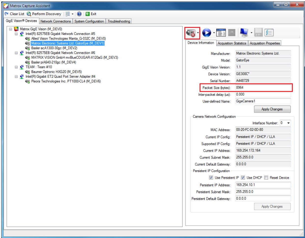
By default, MIL's GigE Vision driver will attempt to negotiate the largest possible packet size with the GigE Vision device. On some networking environments this might not be optimal. This setting can be changed through Matrox Capture Assistant's [System Configuration page](#). Simply select the GigE Vision system type you are using and then set the maximum negotiated packet size and click **Apply**. At the next device allocation, the new packet size will be used.
