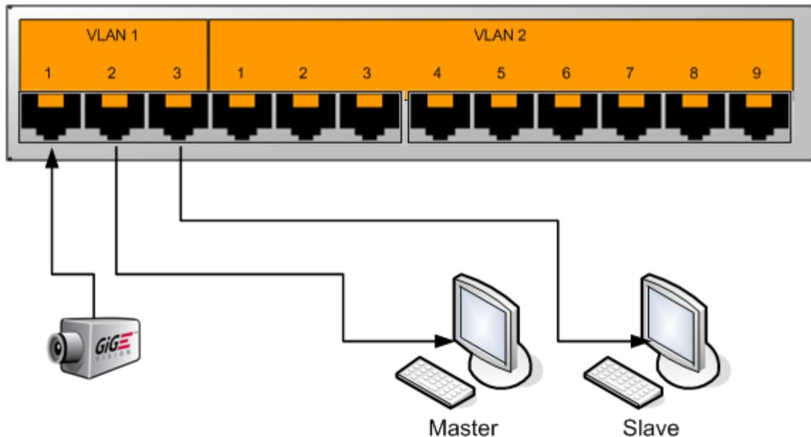
This VLAN partitioning scheme can be used to create other VLANs in order to support additional multicast sources (e.g., GigE Vision devices). It can also be modified by adding ports in order to support more than two destinations per multicast source.
